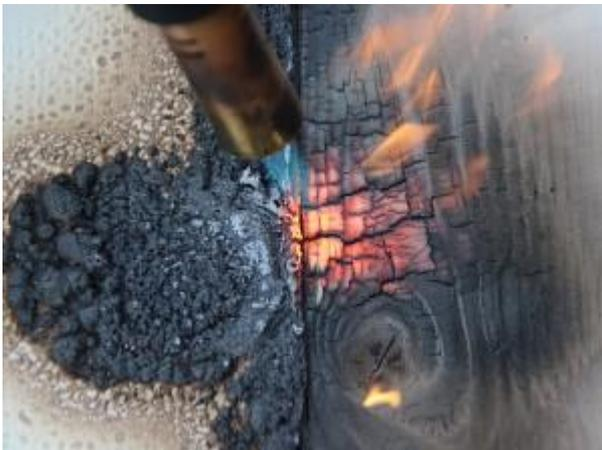
A range of timber substrates can be coated with intumescent paint in order to comply with standards in fire regulations. These building elements include frames, staircases, floors, ceilings, cladding, and doors made of wood or wood derivatives.
